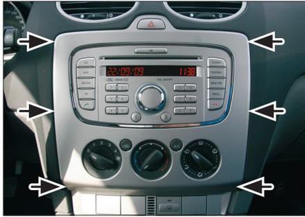
1. Unclip the frame surrounding the OEM-Radio and remove it
