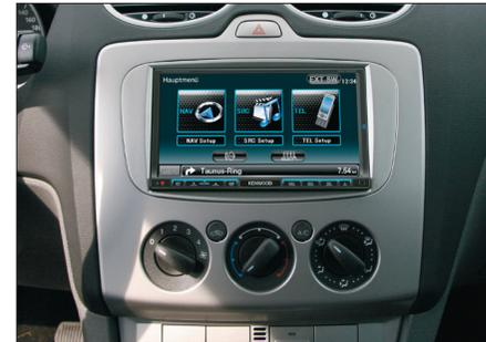
Connect all required circuit points and push the double DIN head unit into the mounting frame until it snaps in
