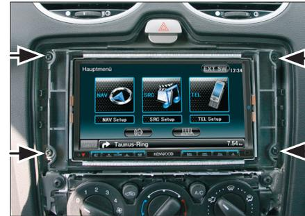
3. Push the head unit with the mounted metal brackets into the metal frame, until it snaps in
