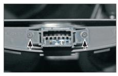
5. Remove the hazard switch fixed to the Hyundai i10 OEM head unit and fix it to the Facia Plate using the 2 original screws (see arrows)
