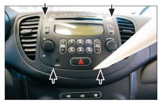
Unclip carefully the center panel surrounding the OEM head unit
