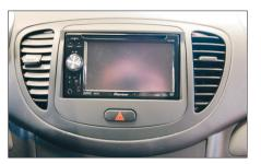
Connect the hazard switch plug with the hazard switch
