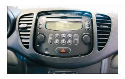
3. Remove the OEM center panel surrounding the OEM head unit
