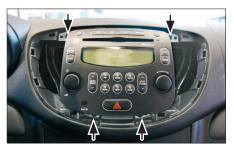
Remove the 4 screws (see arrows) fixing the OEM head unit
