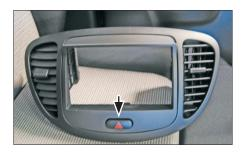
6. Center panel with installed harzard switch
