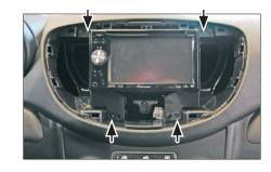
Mount the Double DIN Navigation to the Mounting Frame.
