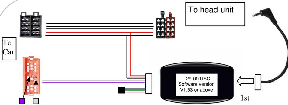
**1-ALWAYS CONNECT THE HEAD-UNIT CABLE ADAPTER 1st before ignition is turned on!**
