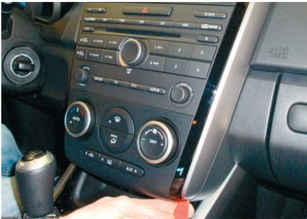
2. Unclip side panels at left and right side
