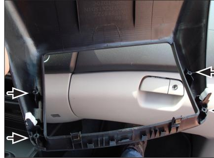
3. Remove 4 screws to disassemble
