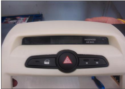
8. Mount hazard light switch and top display to fascia plate
