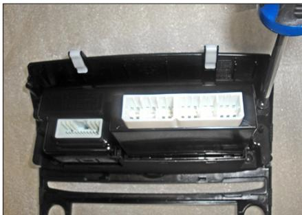
4. Remove hazard light switch and display from OEM bezel
