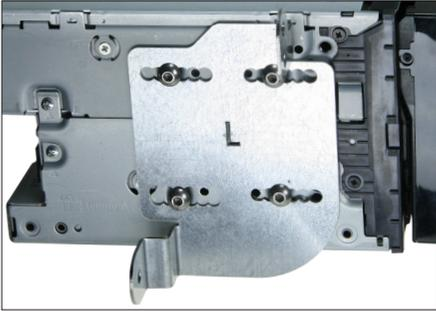
1. Mount brackets to double DIN Navigation as shown in sample photo
