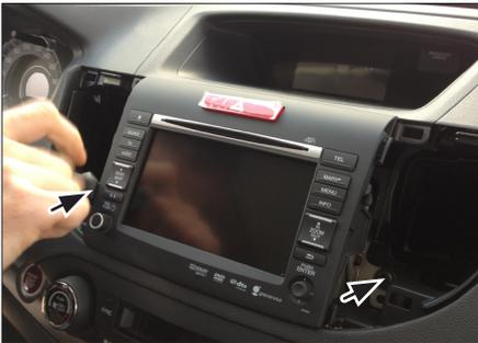
2. Remove screws of OEM head unit (see arrows)
