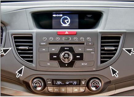
1. Unclip and remove air vents left and right side (see arrows)
