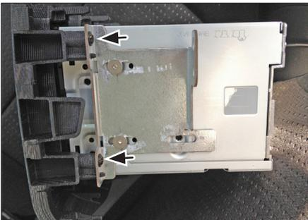
4. Attach metal mounting frames to Double-DIN head unit
