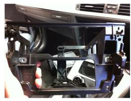
3. Unscrew the plastic sub-dash cage and remove from the dash.
