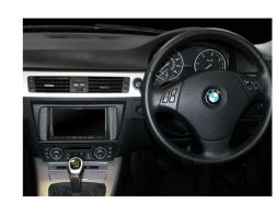
8. Clip the supplied facia and climate control assembly into place over the top of the aftermarket head unit..
