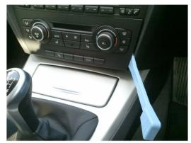
Remove the climate control panel using a panel removal tool.
