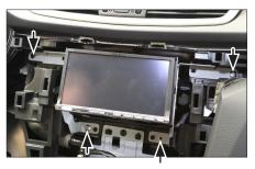
Connect all required circuit points. Place Double-DIN head unit on dash board Fix it with 4 screws
