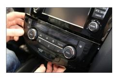
Unclip air condition control unit under OEM head unit
