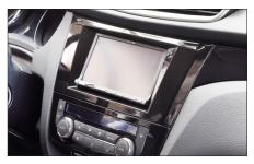
Put clips on the rear side of facia plate. Place facia plate on dash board
